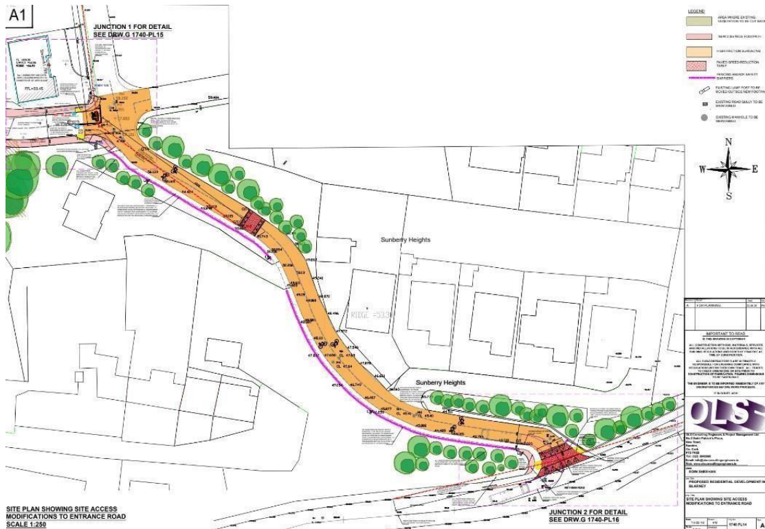
Plate 9 Proposed works to the existing access road
